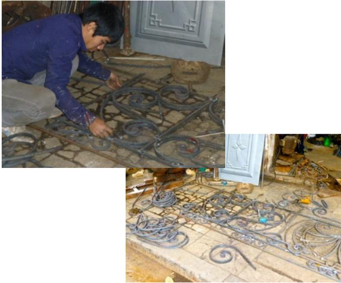
used a tube bender for the scrolls. The home-made bending fork was up to the task. It was a lot of “bend and fit” work but what railing isn’t?
