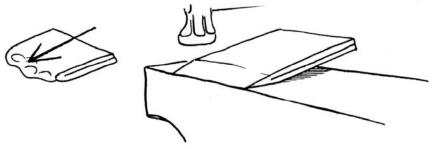
4) If forged in the direction of the fold, that is to lengthen the fold line across the sheet either a curved or straight profile may be obtained. The greater the curve forged in the higher the relief in the unfolded metal.
