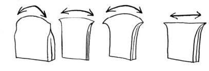
5) The metal is annealed and unfolded gently
