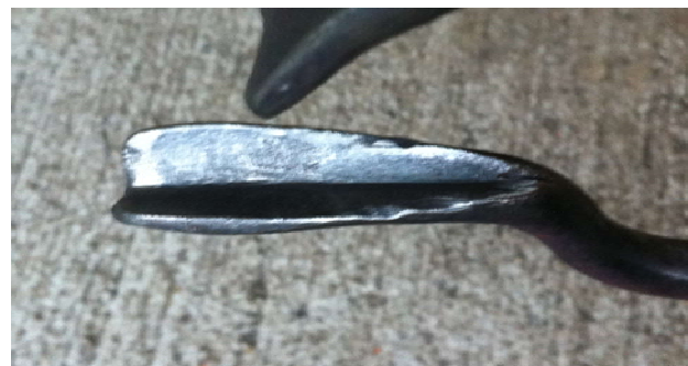
Figure 11: Bottom bit filed to V
