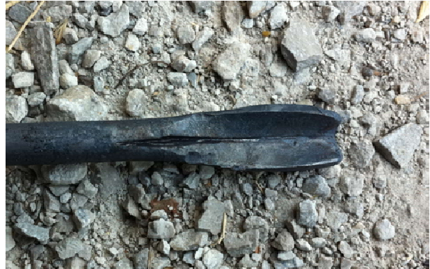
Figure 9: Bottom bit end formed
