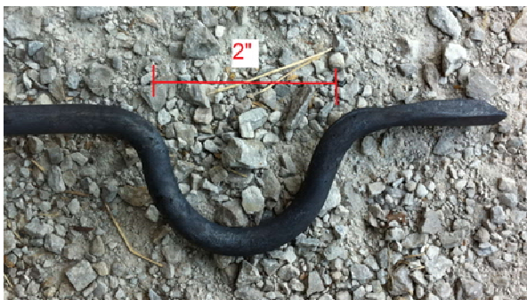
Figure 10: Bottom bit bent to shape
