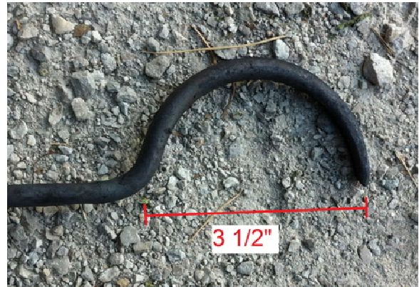
Figure 5: Top bit bent to shape
