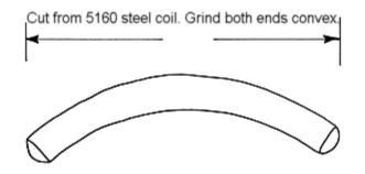
I start the blade by forging an obtuse point on one end. If the stock is forged flat first, the blade will tend to fold down the middle when the point is forged in.
