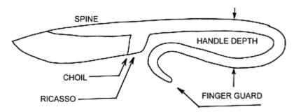
I use a small swage die to round the top of the tang section so that it is more comfortable in the hand. If you are only making one or two knives or you don't want to make a special die, the back of the tang can be rounded on a grinder. This will leave deep scratches that need to be polished out, so I find a swage die to be a good and inexpensive alternative.
