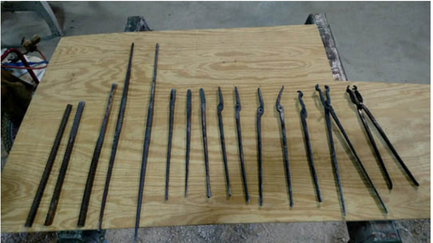
William Bastas once again provided top notch instruction at the May meeting of Balcones Forge. His story board goes a long way in showing the process of taking rebar and turning it into tongs.
