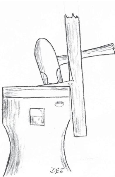
Drawing out the horns – work with square cross section – first one side then rotate 90 degrees and work the other.
