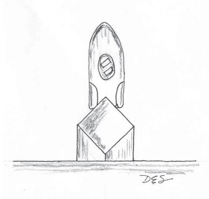
Looking from the side of the anvil setting the eye is done "on the diamond". The second eye will be done by turning the stock 90 degrees and also on the diamond.
