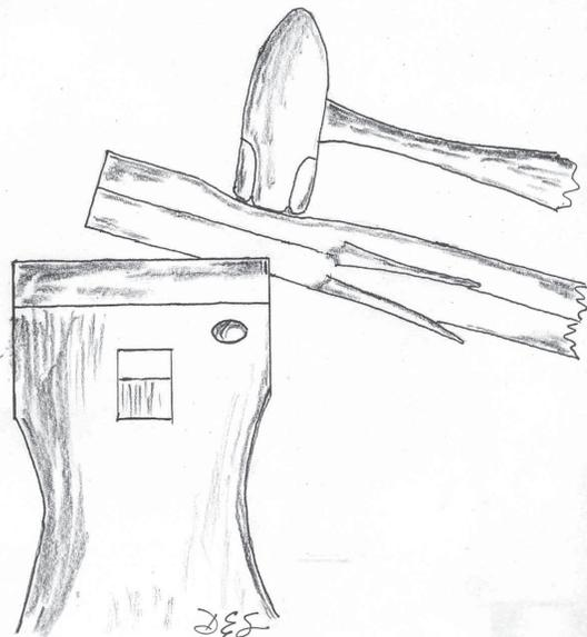
Setting the eye area on the sharp edge of your anvil. Note that the hammer blows are direct to the underside of the head and are "half on half off" the edge of the anvil. This is the first eye; the second one hasn't been started yet.
