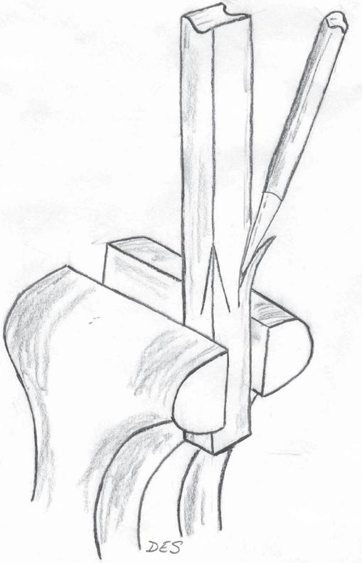
Cutting the horns with "head" clamped in the vise. Keep the hot cut point into the bar; it wants to go vertical on its own.
