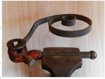
from you. Now, while you stand in a one place, hold the end of the stock at the starting point on the jig, pull the stock towards you until you reach the shops/areas "swing" limit, then ratchet the jig away from you and form the stock around another portion of the jig. At some point the ratchet toggle will need to be flipped to keep the stock pull direction the same – repeat until the scroll is finished.
