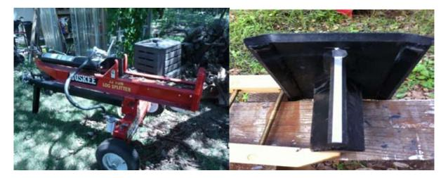
This is the splitter when I started. I only got to use it once to split logs. The first thing I did was to remove the ram and grind the edge of the wedge off. The wedge is an inch wide, so the flat is now about ½ inch across. I found some 1inch plate at a salvage yard and a 4 inch square by 6 inch long solid steel stock that I used for the anvil. I cut the plate and wieldedit to the wedge
