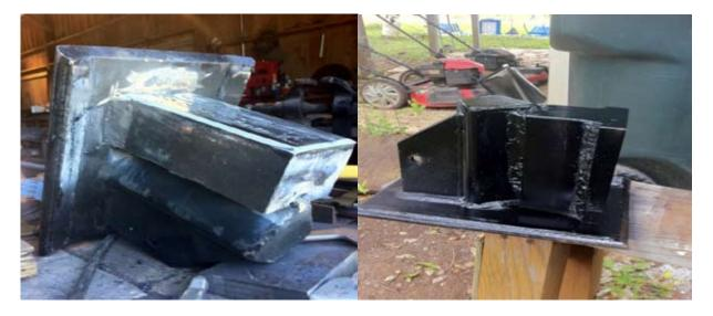
Now the ram is 3 inches wide. But I wanted the ram and the anvil to be the same size, so I added a 1x4 inch plate to the front. This way the die plates could all be cut the same size.
