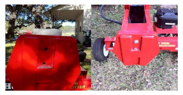
The next thing you need to do is attach the anvil. I did this by drilling two holes in the bottom of the base plate and into the anvil, then threading just the anvil. Now all you need is two 3/8 inch bolts and the base is complete. At this point I trimmed the plate and the anvil up to make everything even
