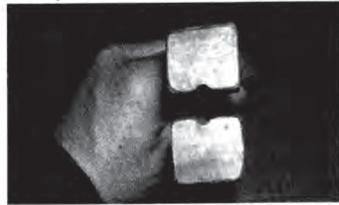
A grooved spring swage matches the other forging tool. A perfect fit can be had if you make this tool first, then use it to forge the pad used in the previous tool.
