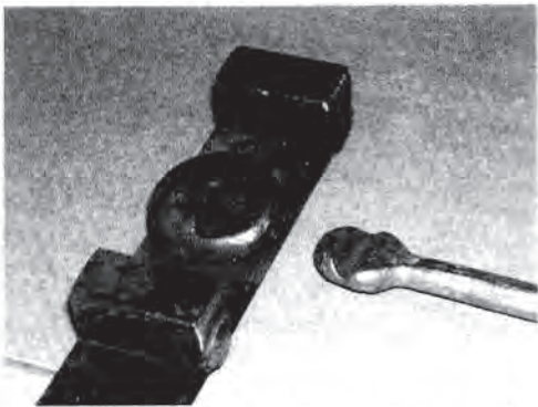
A special tool for flattening the ball ends of the handle. The two blocks on either side are "kiss blocks" that limit the forging to the proper depth.
