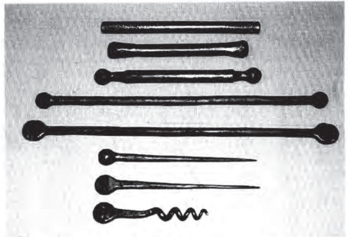
The forging sequence of the corkscrew parts. The top five pieces are the handle at various stages, while the bottom three parts form the center screw.
