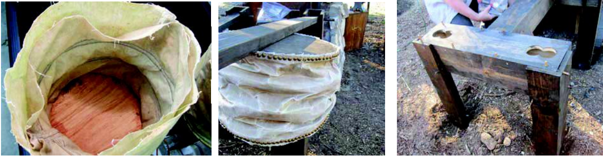
(Left) Inside of bellows showing stay pockets on the inner bag. (Center) Assembled bellows and lifting handle. (Right) Cross plenum showing twin three inch diameter holes for air discharge from the bellows. Note the dowels holding the supporting legs in place.
